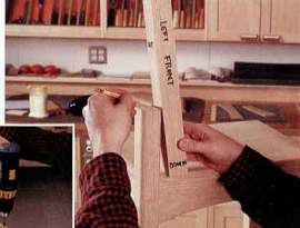
Figure 5: Hold the back posts as shown above on the assembled base with the seat in place. Then locate the bottom of the seat using the tops of the front legs as guides. Later, (left) you'll attach the armrests with glue and screws.
