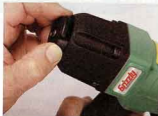
Each time you fire a brad, a puff of air is exhausted from the nailer. On the Grizzly (and others), you can rotate the top-mounted exhaust to direct the air away from your face.
