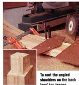
To rout the angled shoulders on the back legs' top tenons, I made a jig that registered the angles and clamped to both legs, so I could mill them in one setup. A rub collar on my router followed the angled jig shape to cut the shoulders. Flip the legs over in the jig to make the second set of angled shoulders.
