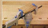
Securing your stock is an important task. You also need to be able to spin the stock around easily ... it allows you to easily pull the cut towards you.
