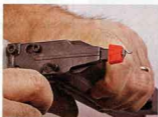
Sometimes a jam-up occurs. Some nailers, like the Makita (above), use an Allen-wrench to open the drive cover. Others simply pop a latch to open the cover and clear the jam.
