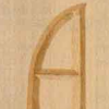
Remove the paper and sand the surface smooth. If you're painting the carved area ... leave the paper on.
