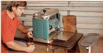
The Makita 2012NB benchtop planer is clamped down to a low work table, preparing it for planing a couple of rough boards chainsawed from backyard harvested logs.
