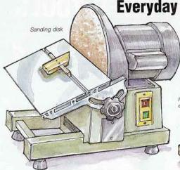
Hardware gauge fits existing slot in table.
