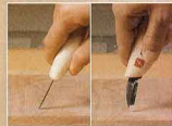
Knife angle is the key to achieving uniform carved letters. About 65° is where you should start. Near perpendicular is most effective as you look at the side of the knife.
