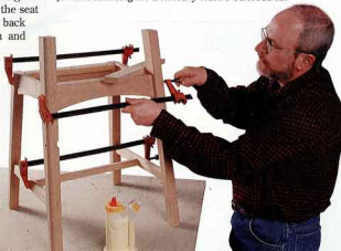
Figure 4: Glue and clamp the base parts together on a flat surface. Laying a board across the tops of the side and front aprons will ensure that the front apron is at the proper height.
