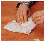
By wrapping a center pad of trace cloth with a well-washed piece of linen, the author creates the perfect application pad.
