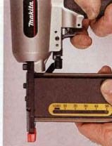
Makita has a feature that controls the safety reset with the trigger of the nailer. Also note the window to see if brads are loaded or not.
