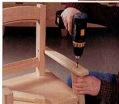
Figure 5: Hold the back posts as shown above on the assembled base with the seat in place. Then locate the bottom of the seat using the tops of the front legs as guides. Later, (left) you'll attach the armrests with glue and screws.
