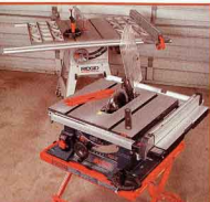
Set up on its folding workstand is the Bosch 4000 benchtop table saw. Lighter and smaller than the rigid contractor's saw behind it, the Bosch has the same maximum cutting depth and 24" rip capacity.
