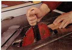
How forceful do you have to be with your arbor nut? Kelly Mehler has tips for getting it just right: not too snug, not too loose.
