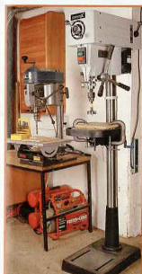
Ryobi benchtop; Delta variable speed. Both models have infinitely-selectable variable speed, a feature that makes them practical and versatile for drilling a variety of materials.
