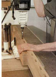
The back slats fit into individual mortises in the back rail. A hollow chisel mortiser is the perfect tool for this repetitive chopping task.
