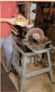
For sanding large flat or convex parts, nothing beats the large capacity and power of a stationary sander, such as the Delta Sanding Center shown here.
